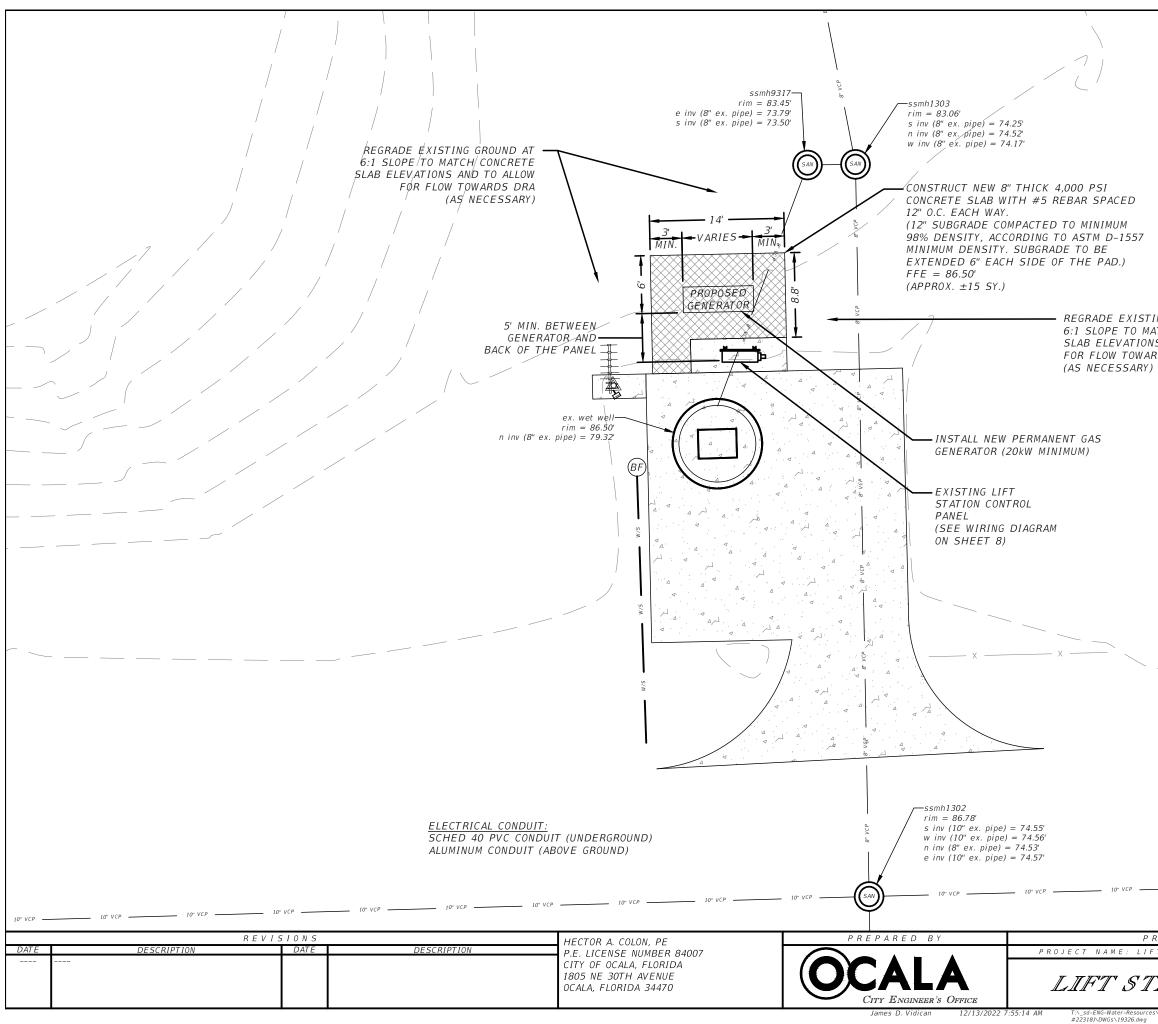
REGRADE EXISTING GROUND AT 6:1 SLOPE TO MATCH CONCRETE SLAB ELEVATIONS AND TO ALLOW FOR FLOW TOWARDS DRA 10" VCP -----PROJECT NO. 19326 SHEET PROJECT NAME: LIFT STATIONS #9 & #22 IMPROVEMENTS NO. LIFT STATION #22 PLAN 6
